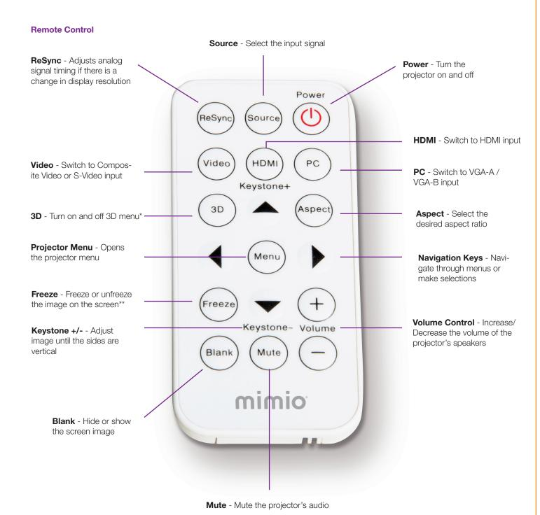
\*Mimio does not provide 3D content; DLP Link 3D and HDMI 1.4a 3D supported.
